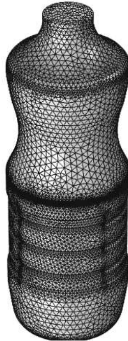
Mesh of surface 23 thousand triangles
