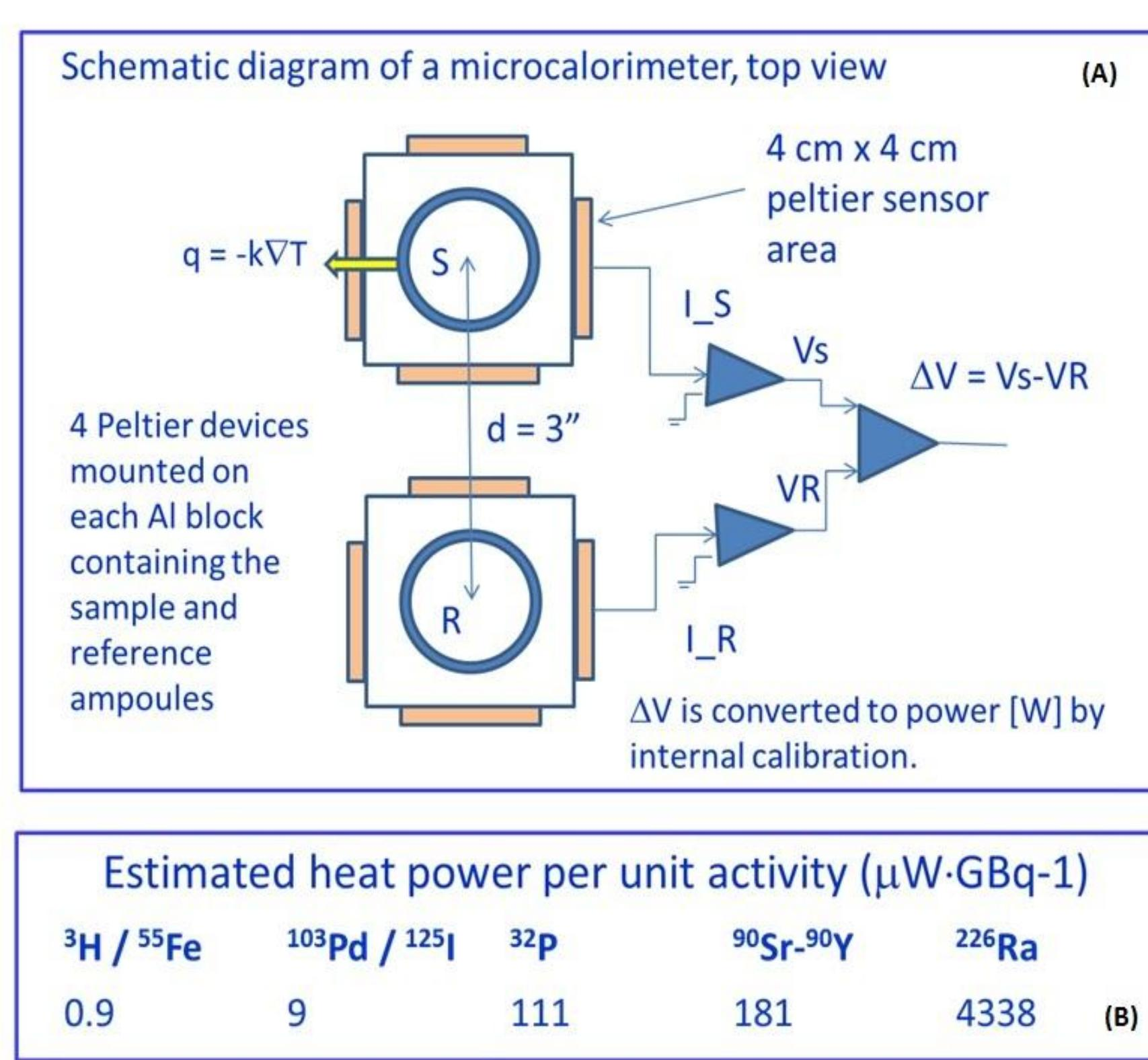
**Figure 1.** Principle of operation of a microcalorimeter (A) and radioactive decay power (B).
