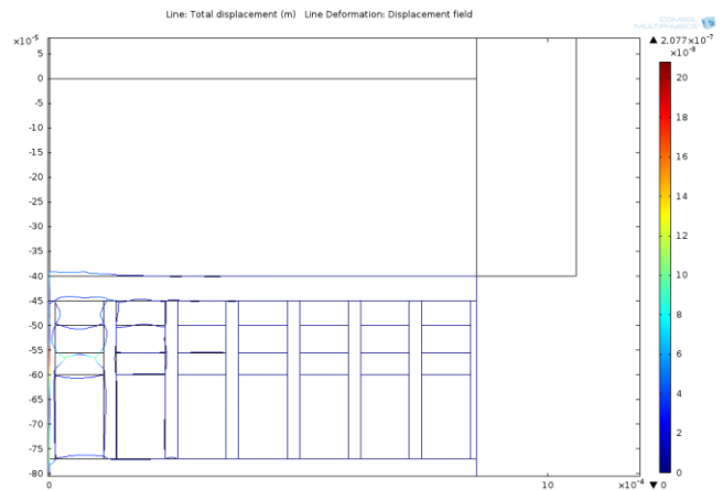
Figure 9: Deformed shape at 8MHz, on axis element excited.
