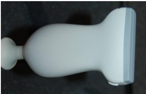
Figure 5: Complete probe head, with silicon lens and plastic covers.
