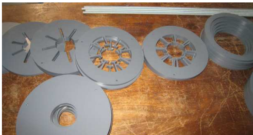
Figure 2. Resonator plates for the test section.
