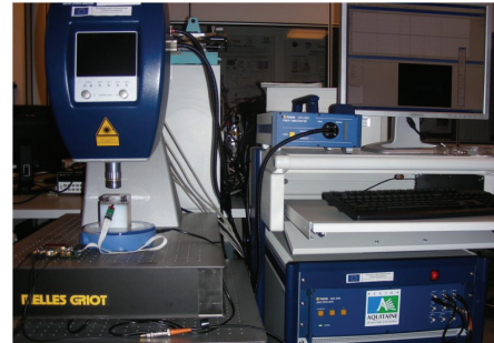
Figure 3. Photo of the vibrometer (left) with data processing (right) .
