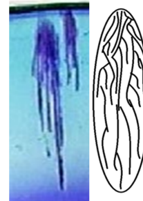
Figure 2: Single water tree and ellipsoid representation
