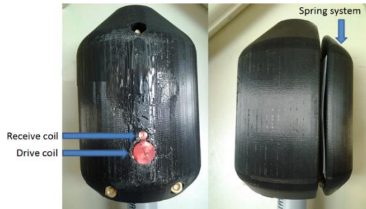
Figure 2: A photograph of the experimental PEC probe showing its basic components.
