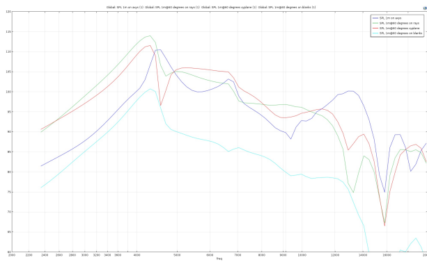
Figure 4: Simulated tweeter response with corresponding 60 degrees off axis response
