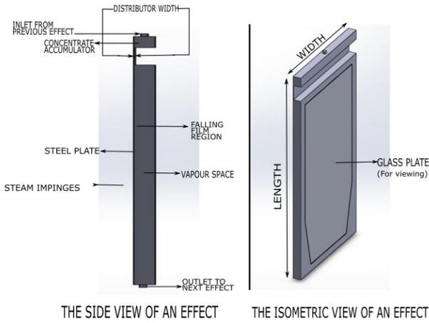
Figure 1: Illustration of the geometry of an evaporator effect.
