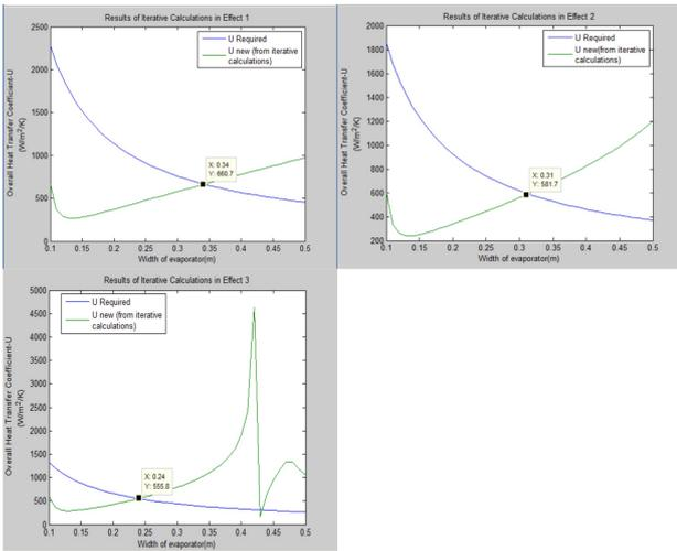
Figure 2: Graphical results of the iterative design procedure for sizing the evaporator effects.
