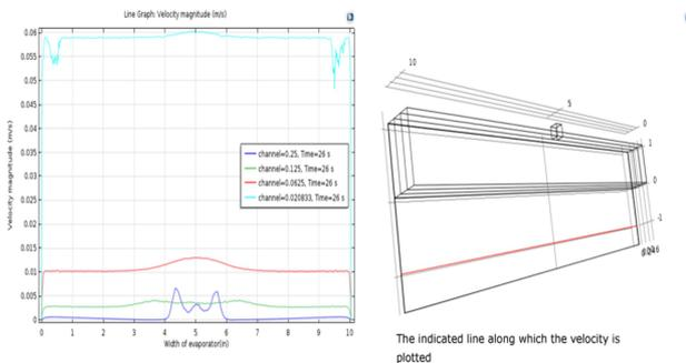
Figure 3: Velocity profiles for different geometries of the distributor channel.
