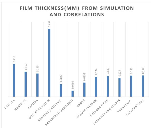
**Figure 4:** Graphical comparison of film thickness(mm) obtained from various correlations with the COMSOL® Simulations in the first effect.
