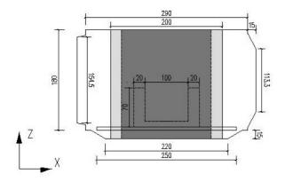
Figure 3: Fig.1 Geometry of the 3-D microwave oven: x-z plane view
