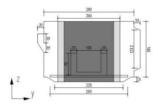
Figure 1: Fig.1 Geometry of the 3-D microwave oven: y-z plane view
