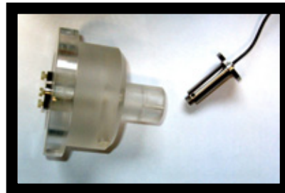
Figure 1. Dummy cavity made in plexiglass together with a capacitive sensor used to measure cavity expansion during preliminary tests.
