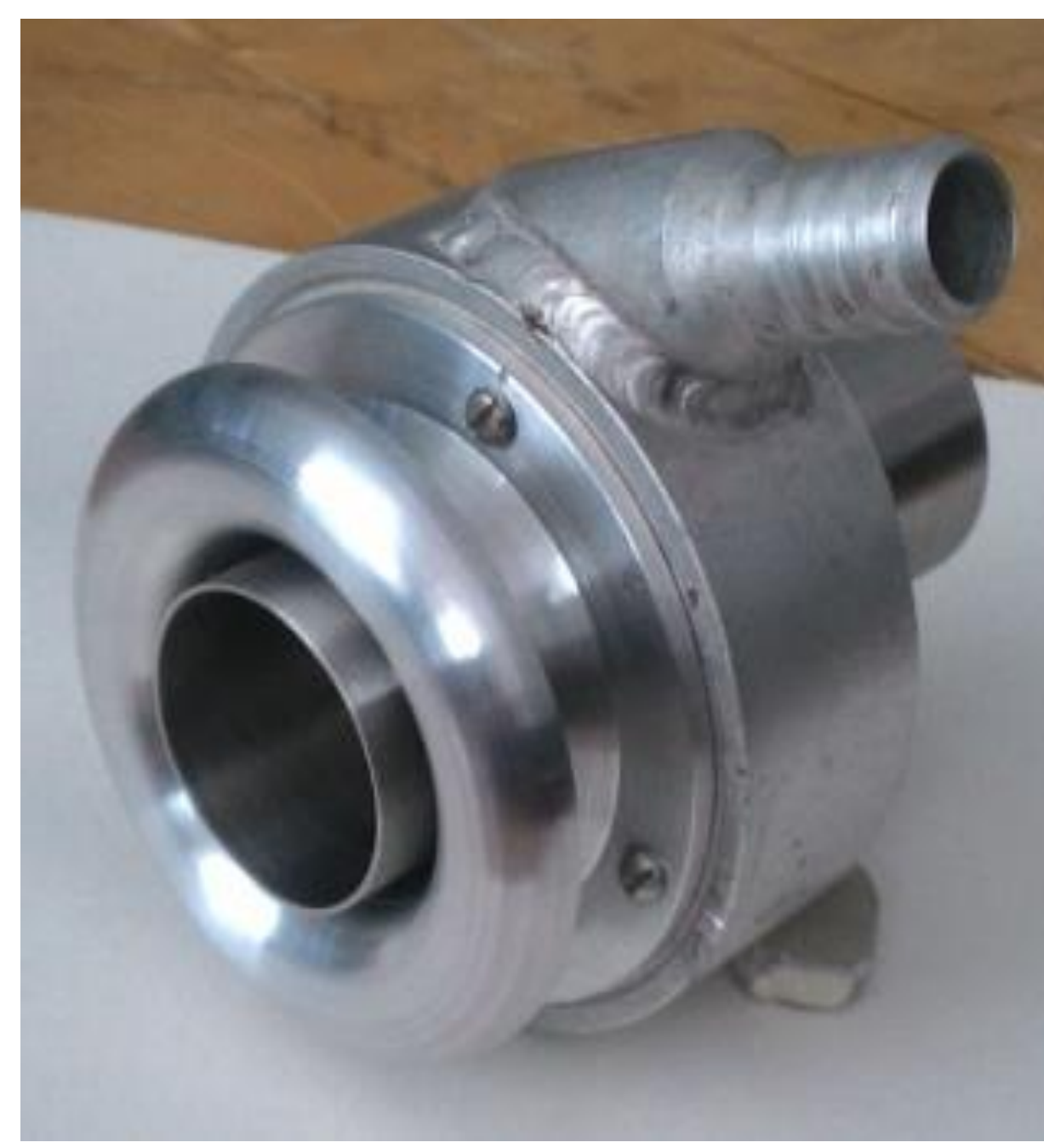
Figure 2. The unit for the focusing of the extraction flow [1]
