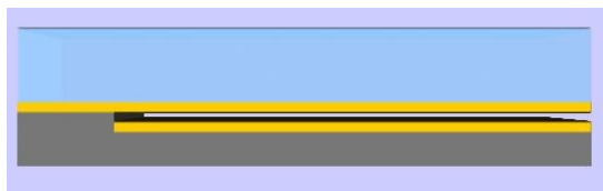
Fig. 8 (f) Bonding of both substrates using Pyrex bonding
