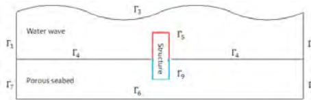
Figure 1. Locations for specification of boundary condition.
