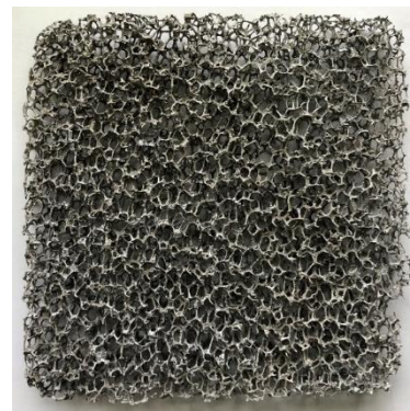
Figure 1. An open-cell metal foam.
