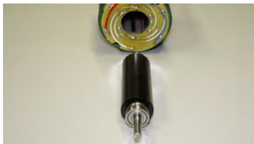
Figure 2 Synchronous machine (DUT)
