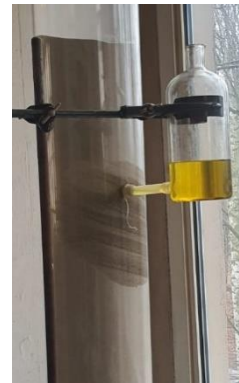
Figure 6b. Laboratory model illustrating diesel saturation front in 20-hours of imbibition implemented as mid-column experiment.
