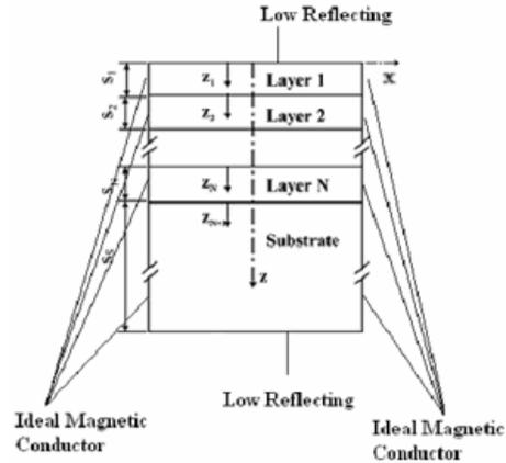
**Figure 2:** Thin film, TCO and glass substrate optical model.
