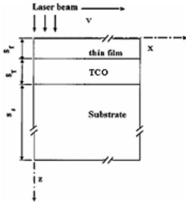
Figure 1: Sketch of the thin film and the TCO layer on glass substrate.
