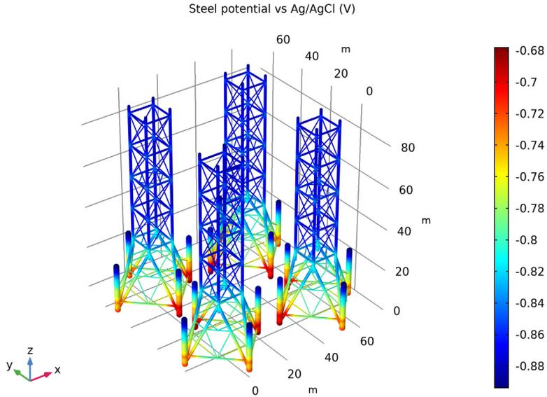
Figure 4: Potential distribution on the steel structure vs an Ag/AgCl reference electrode.
