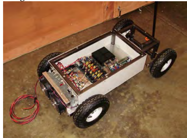
Figure 1. Test cart including wireless power amplifier, heat sink, fans and ducts.
