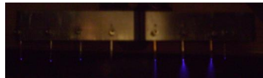
Figure1. Corona light in a needle tip-plate configuration for different needle materials: gold, aluminum, silver, steel, diamond coated steel and tungsten. The grounded plates all are made of copper.
