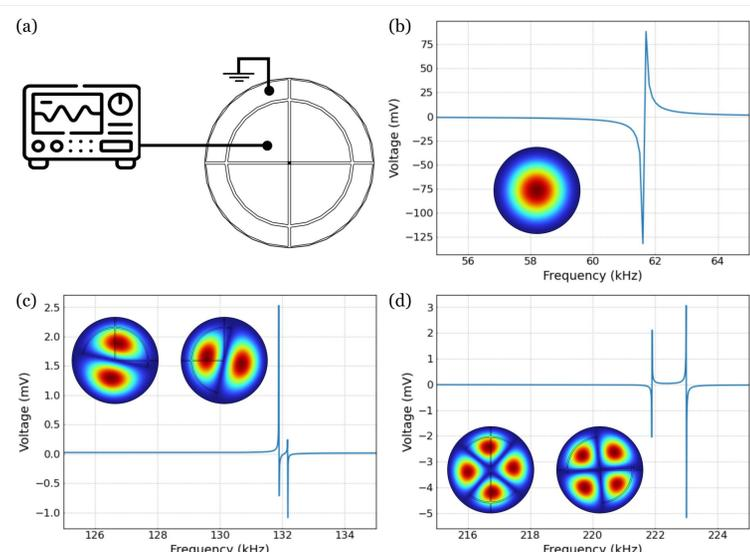
FIGURE 2. (a) Representative electrical connections for voltage measurement. (b), (c), (d) Voltage output for transverse modes
