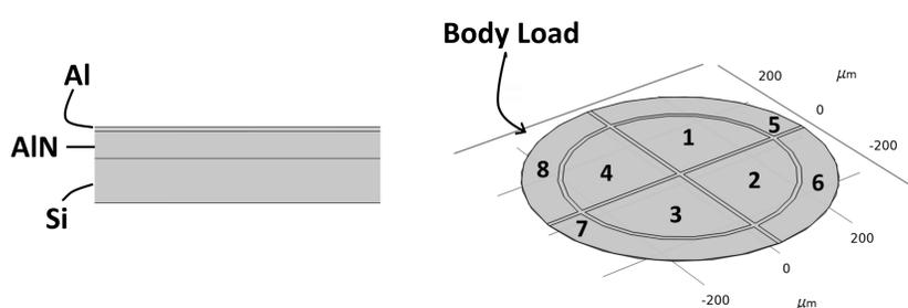
FIGURE 1. Left: Material stack used for the MEMS-based AE detector. Right: 8-electrode configuration on a single membrane with the body load applied to the entire device.
