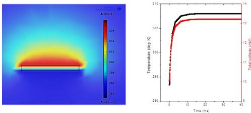
**Figure 1:** Left: Steady-state temperature distribution in a 60  $\mu\text{m}$   $\text{Bi}_2\text{Te}_3$  under a 10mV pulse of 0.5 s length. Right: Temperature and voltage as function of time for same applied voltage pulse.
