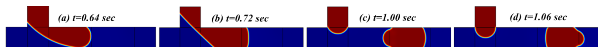
Figure 3. Deformation in a ‘plug’ patten is observed when it passes through an applied field (500 Volts) at different time intervals.
