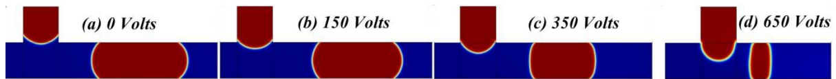
Figure 2. Effect of voltage on the plug size. Here the electrodes are placed across the entire length of channel (L) from T-junction.
