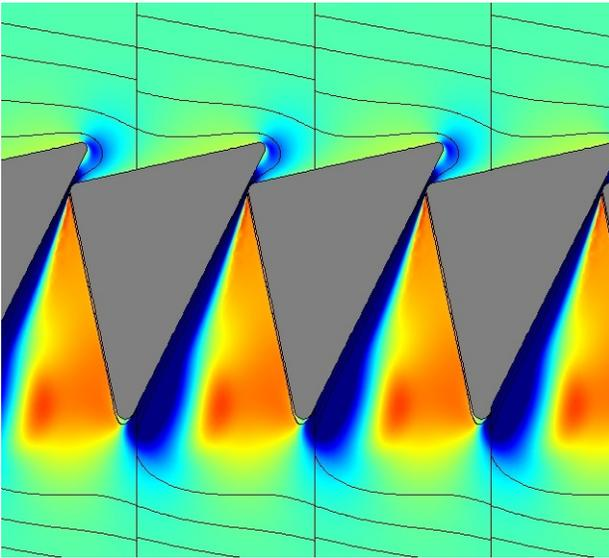
**Figure 3:** Pulsating flow around the screen barrier
