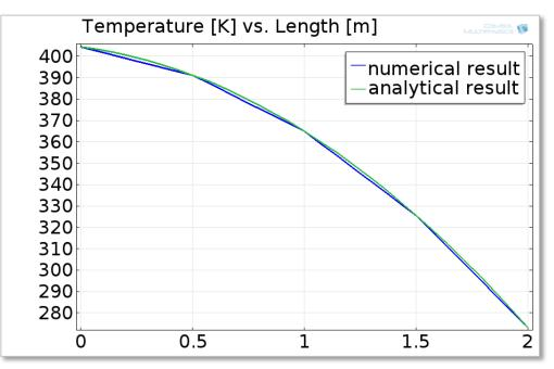
Comparison between the numerical (4 elements and linear shape functions) and the analytical results for  $k = 76,2 \frac{W}{m \cdot K}$ , L = 2 m,  $Q = 4000 \frac{W}{m^3}$ ,  $q_0 = 1000 \frac{W}{m^2}$ , and  $T_0 = 273,15 \text{ K}$ .
