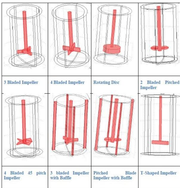
**Figure 1:** Different types of impeller geometries.
