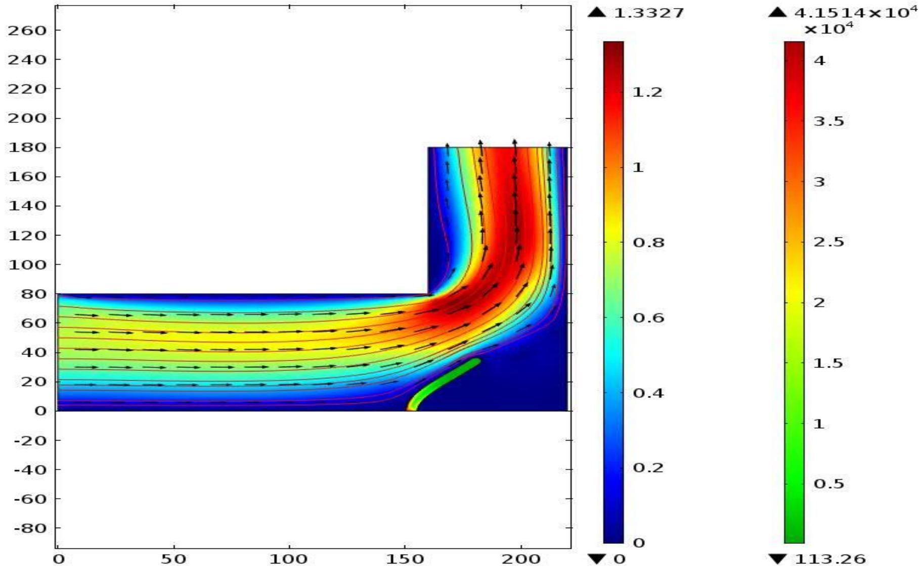
Time=4 s Surface: von Mises stress (N/m<sup>2</sup>) Surface: Velocity magnitude (m/s) Arrow Surface: Velocity field (Spatial)
