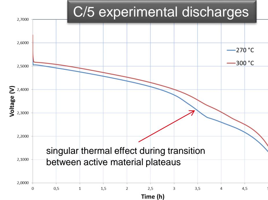
➔ The model is validated in terms of operational temperature. Temperature does not have a significant effect on the voltage curves
