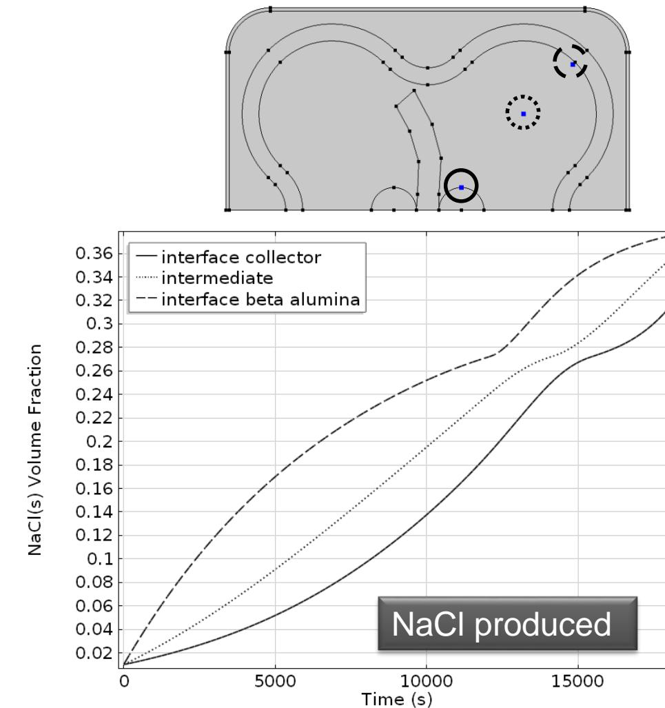
→ a diffuse reaction front moves from the beta alumina towards the central collector
