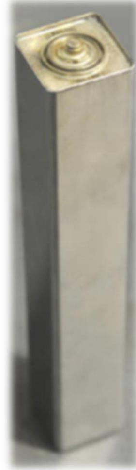
Fe based solution Na-FeCl<sub>2</sub>
