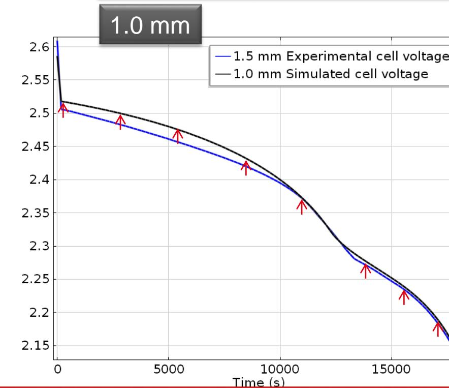
→ As expected, the model predicts less overall polarization with a thinner solid electrolyte
