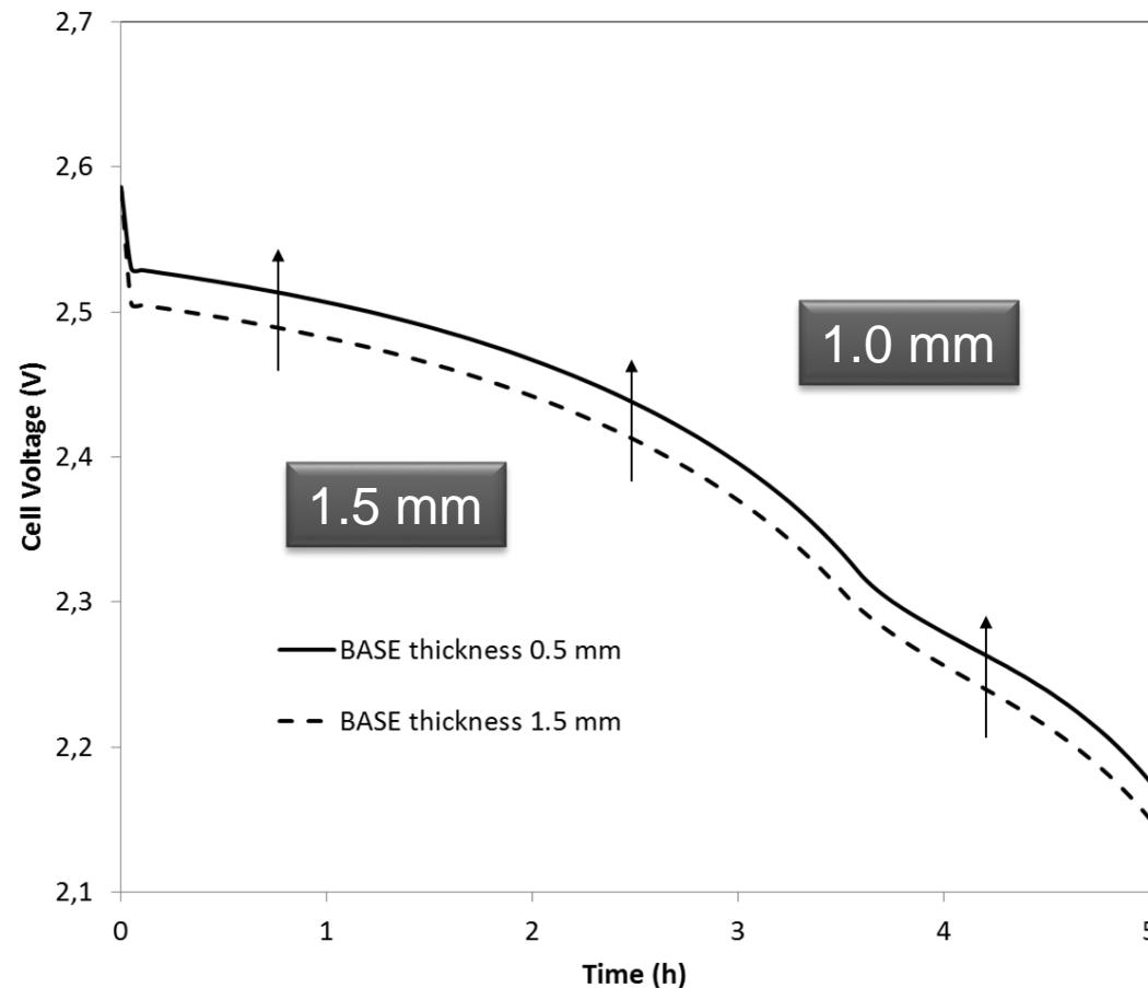
Only the thickness of the beta alumina has been changed between simulations
