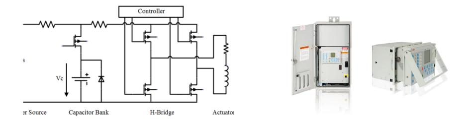
The Electromagnetic actuators of ABB 3-phase GridShield® recloser are powered by suitable Electronic Control Units enabling safe Closing Opening Closing cycles all over the temperature ranges
