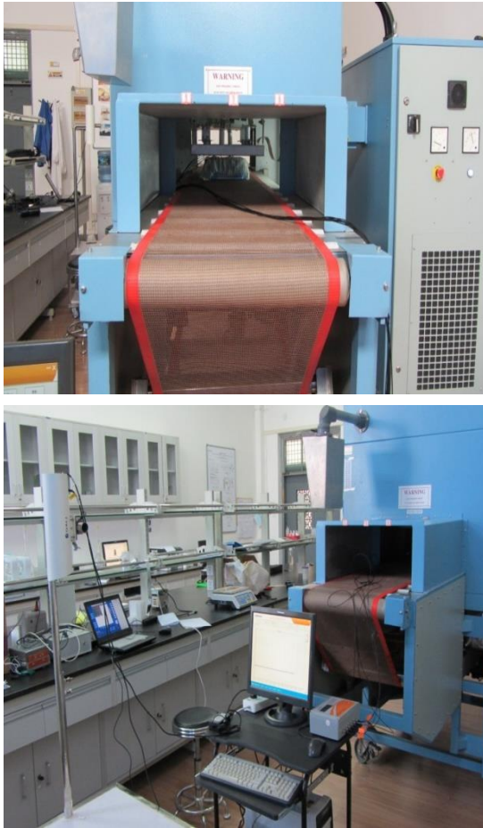
Fig. 1. 6 kW, 27.12 MHz free-running oscillator RF heating system and boundary conditions of RF system used in simulation.
