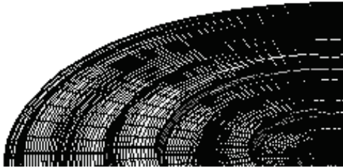
Figure 1. Swept mesh for the circular plate.
