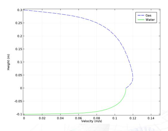
Fully developed velocity profile mapped to reactor
