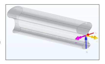
\* 5. A one-meter cantilever beam is subjected to a tensile load of T=300 KN exerted at the center of the free-end cross section of the beam. What would be the maximum displacement point of a cross section, 50 cm away from the fixed end, if a) beam has a vertical rectangular cross section, b) beam has a horizontal rectangular cross section? The wireframe schematic of the beam along with the undeformed cross sections for each case are presented below.
