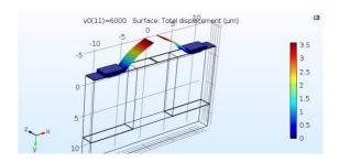
Figure 2: Displacement of membrane on application of electric filed.
