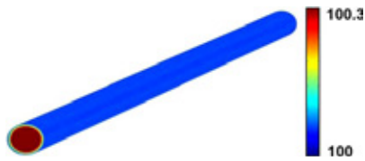
Figure 8. Temperature [ ^\circ\text{C} ] distribution in the insulated wire at I_{\text{rms}} = 4 \text{ A} calculated with electro-thermal simulation.
