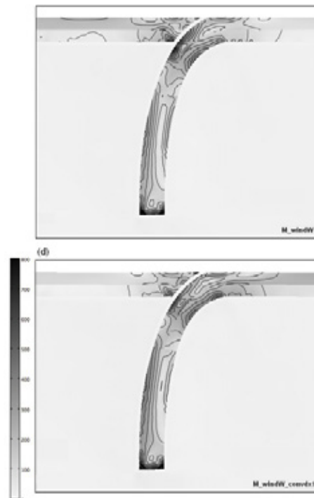
Figure 5. Von Mises stresses (in MPa) calculated for models with Marianas-like geometries and characterised by mantle flow opposite to the direction of subduction (top) and by mantle flow and convergence (bottom).
