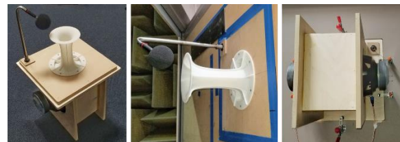
Figure 7. Test box setup with two 10-inch drivers. Left: Box before mounting. Middle: Box with port mounted inside hemi-anechoic chamber. Left: View from outside hemi-anechoic chamber.
