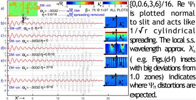
is plotted normal to slit and acts like 1/√r cylindrical spreading. The local s.s. wavelength approx.  $\lambda'_{s}$ (e.g. Figs.(d-f) insets with big deviations from 1.0 zones) indicates where  $\Psi_n$  distortions are expected.
